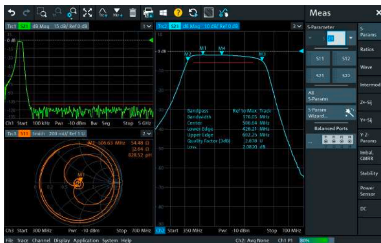
Characterization of a bandpass filter.
