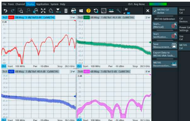
Real-time S-parameter measurements with uncertainty bands.
