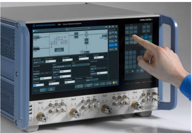
Control of the R&S®ZNA via touch panel. Users benefit from all-in-one dialogs, which provide a clear overview of all key parameters and help to keep track of the overall measurement configuration.
