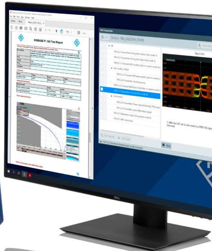
Automated Auto Ethernet compliance test
