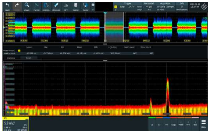
The high bandwidth of the R&S®RT-ZPR power rail probes allows you to capture high-frequency noise components
