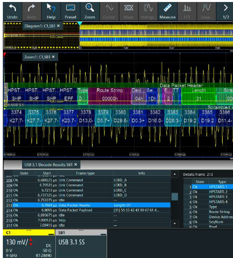
Clear display of decoded data in the waveform and in the decode table
