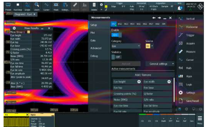
Select from an advanced set of automated Eye measurements
