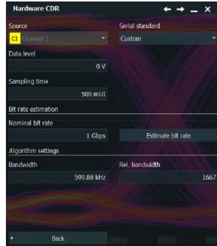
The configurable HW-CDR of the R&S®RTP supports data rates up to 16 Gbps for data eye analysis.
