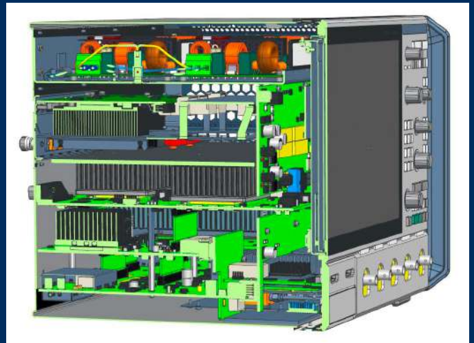
Extremely compact layout of the R&S®RTP
